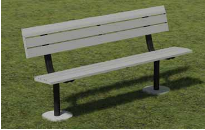
Model SCXB/G-6/TA Embedded Mount Bench with black powder coated frames, 6 ft. long with gray thermo-plastic coated steel channel seat and back.
