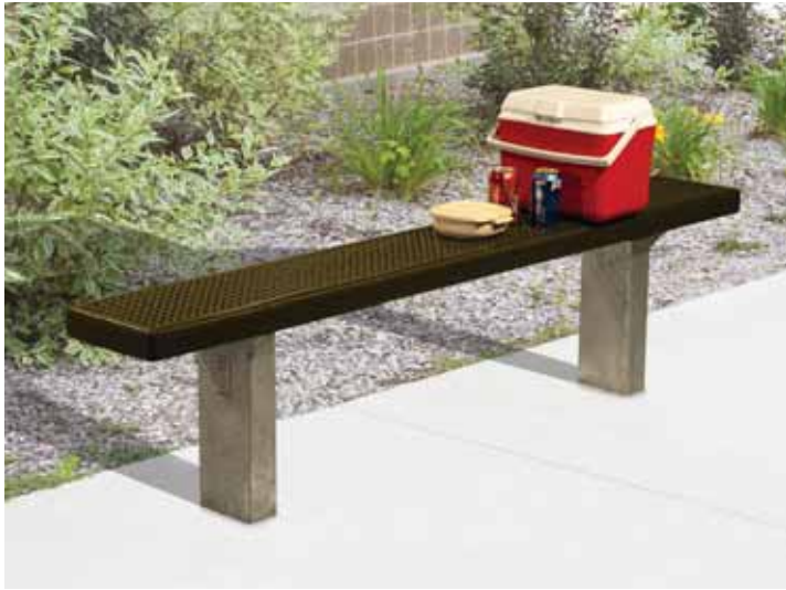
Model APB/G-6HW10 Embedded Mount Bench with Hot Dip Galvanized Frames, 6 Ft. long with 10" wide Brown Thermo-plastic Coated Perforated Steel seat.
