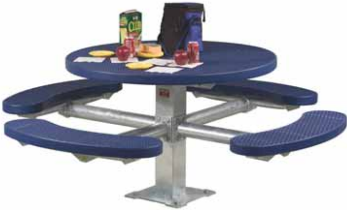
Model T404/G-4DU Surface Mount, Single Pedestal, Round Table with hot dip galvanized frames, with blue D-Type thermo-plastic coated 4 ft. dia. expanded steel top and curved seats.
