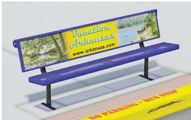
Model B412/CB-8HU Sign Bench, bolt-down surface mount, black powder coated frame, 8 ft. long, blue thermo-plastic coated perforated steel, seat and sign frame.
