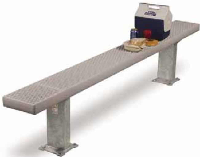
Model APB/P/G-8VA10 Surface Mount Bench with Hot Dip Galvanized Frames, 8 Ft. long with 10" wide Gray Thermo-plastic Coated V-Type Expanded Steel seat. Shown with optional base plate for surface mounting.
