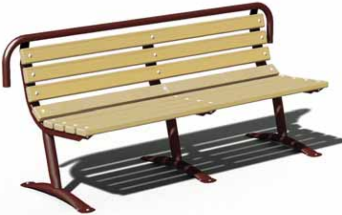
Model B110C/CW-6TP24 Accessible Surface mount Contoured Bench, 6 foot long, with Brown Powder Coated Frames and 2" x 4" Treated Southern Yellow Pine Seat planks
