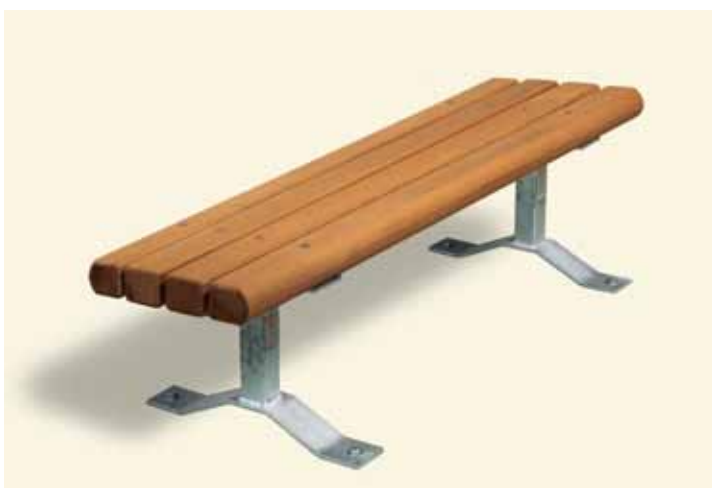
Model PWB/G-6IB34 6 Ft. Portable/Surface Mount Bench with Hot Dip Galvanized Frames and Indonesian Balau Wood 3" x 4" timbers.
