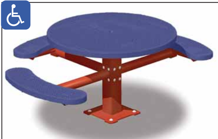
Model T403/CR-4RU Surface Mount, Single Pedestal, Round Accessible Table with red powder coat frames, with blue R-Type thermo-plastic coated 4 ft. dia. perforated steel top and curved seats.
