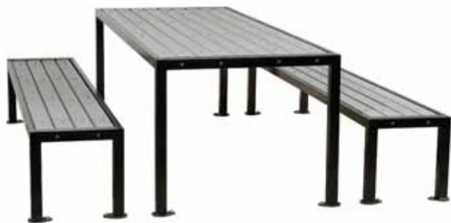
Model T702/CB-8PA surface mount wheelchair accessible square frame table with black powder coated frames, 8 ft. long with gray recycled plastic top and seats.
