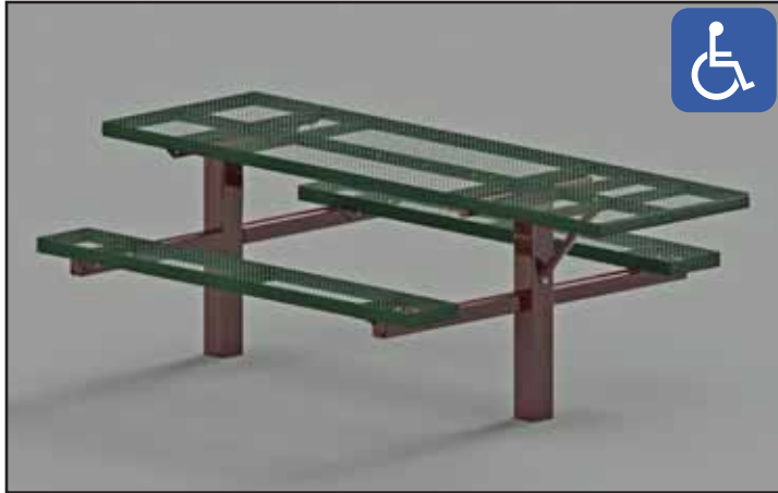
Model TPT/CW6DN/E embedded mount twin pedestal wheelchair accessible table with brown powder coated frames, 6 ft. long seats with 8 ft. long top extended one end, with green thermo-plastic coated expanded steel top and seats.
